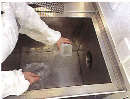
Figure 4: Bail out any collected water into a clean bag for disposal outside the clean room.
