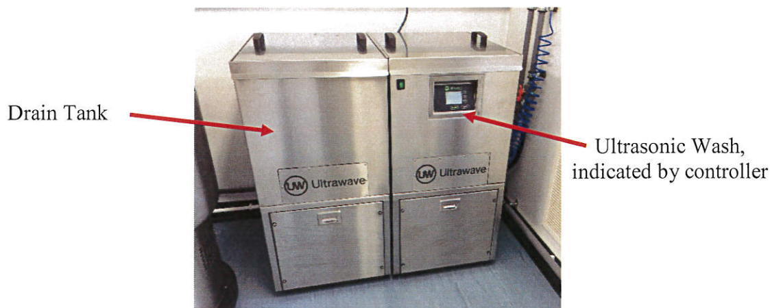
Figure 1: The arrangement of the Ultrasonic Cleaner and drain tank.
