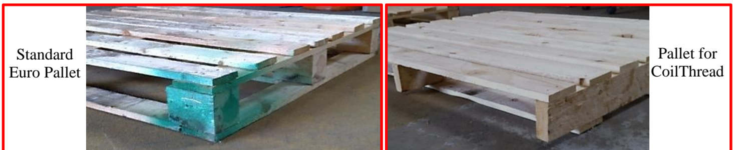
Figure 28: Standard Euro pallet with access from all sides, NOT Acceptable for CoilThread shipments, use pallets with access from only two sides.
