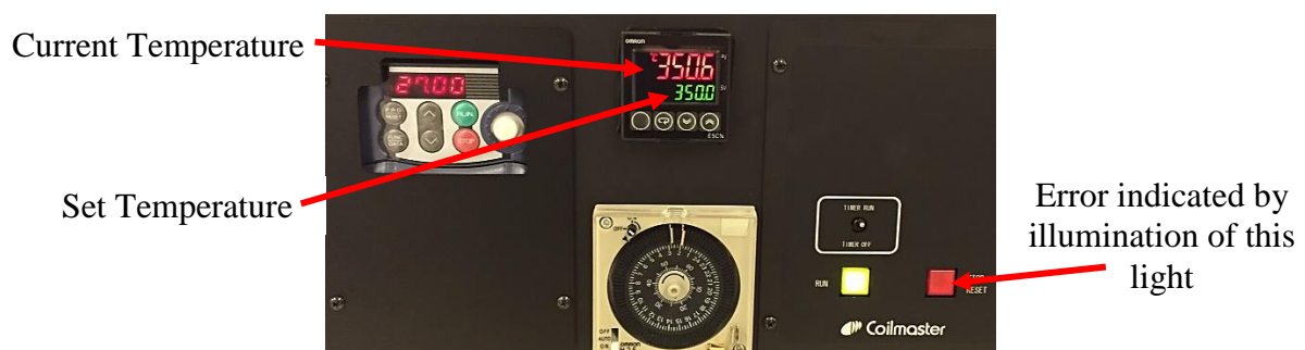
Figure 2: Example of a Temperature control panel.
