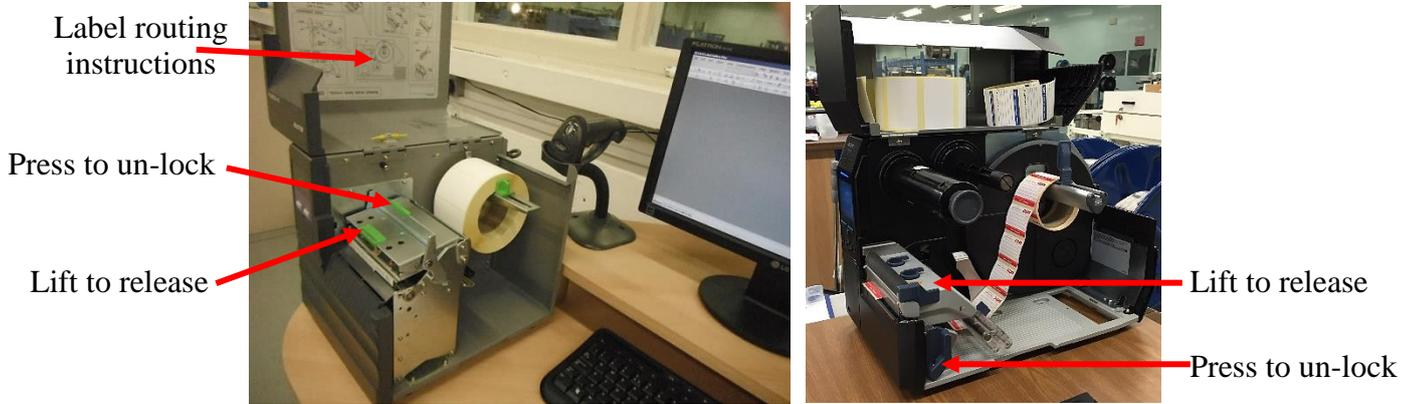
Figure 1: Examples of label print work station.
