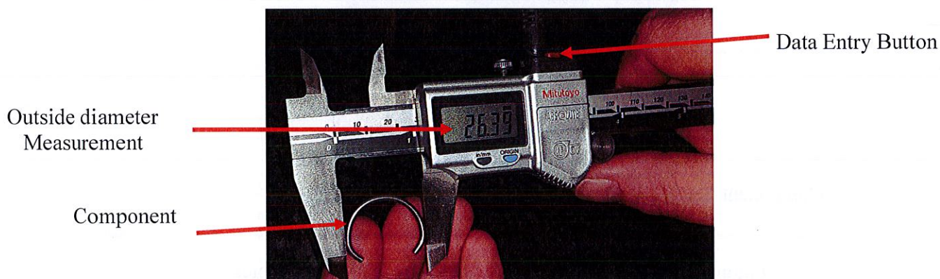
Figure 8. Outside diameter being measured by Vernier callipers
