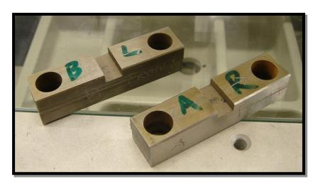
**2** Place wire guides "A" into support "A" and wire guides "B" into support "B".
